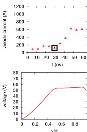
Figure 2: The phase space (upper right), voltage (lower left), and electric field (lower right) at 30ns after the start of electron flow. Ions are shown in blue. For reference, we also show the time history of the anode current (upper left), with the relevant time indicated with a square.
