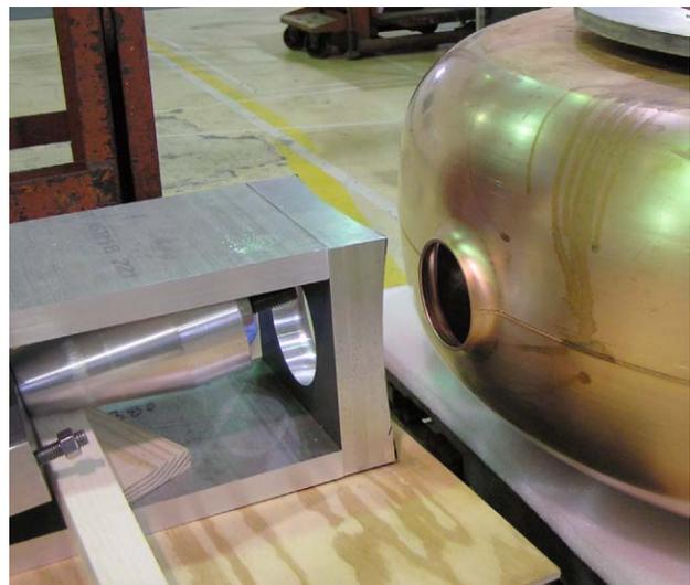
Figure 6. Port pulling after e-beam annealing.
