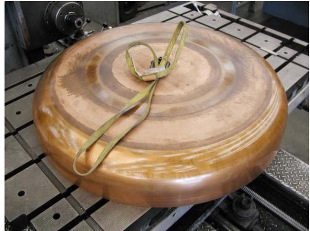
Figure 1: Spun cavity half-shell.
