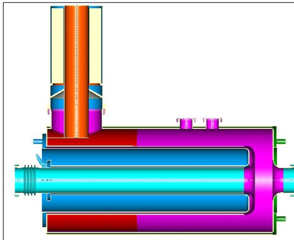
Figure 5: (Color) Mechanical design of the new cavity. The accelerating gap is shown on the right. The tuner is shown on the top left.
