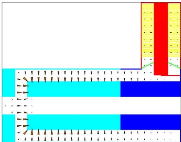
Figure 3: (Color) Longitudinal cross section of the cavity system with the electric field of the fundamental mode shown. The driver located 90 degrees from the tuner is not shown. The ceramic window separating the tuner and the cavity vacuums are also included in the model.
