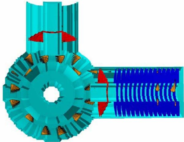
Figure 2: (Color) Three dimensional simulation model showing the transverse cross section of the cavity (on the left with beam pipe hole), tuner (on the right) and the driver (on the top). The magnetic field of the fundamental accelerating mode is also shown.
