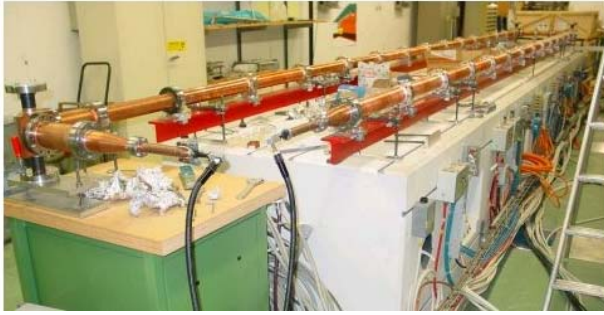
Figure 4: The over-moded line with three mitred bends and converters to WR-34 waveguide.
