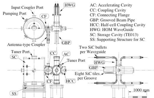
Figure 1: Top, front and side views of the ARES cavity for KEKB.
