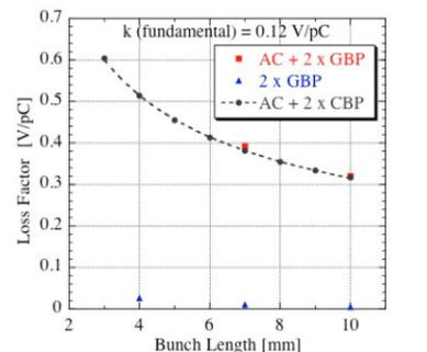
Figure 4: Computed loss factors are plotted as a function of bunch length: rectangles for the whole damped structure, triangles for the two grooved beam pipes only, and circles for a simplified axially symmetric cavity with circular beam pipes attached to both end plates.
