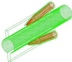
Figure 6: 3D model of a twofold grooved beam pipe loaded with two bullet-shaped SiC absorbers.
