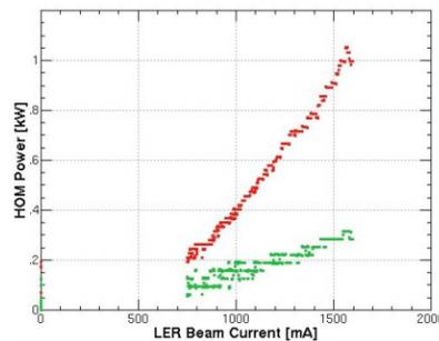
Figure 3: Results of HOM power measurements at the KEKB LER. The upper plot shows the power dissipation in the waveguide load consisting of two bullet-shaped SiC absorbers, and the lower shows the grooved beam pipe load consisting of eight SiC tiles.
