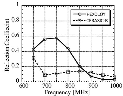
Figure 7: Reflection coefficients computed for the HOM load model in Fig. 6: open circles for HEXOLOY and open rectangles for CERASIC-B.
