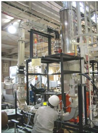
Figure 5: New HOM-load test bench under tuning.
