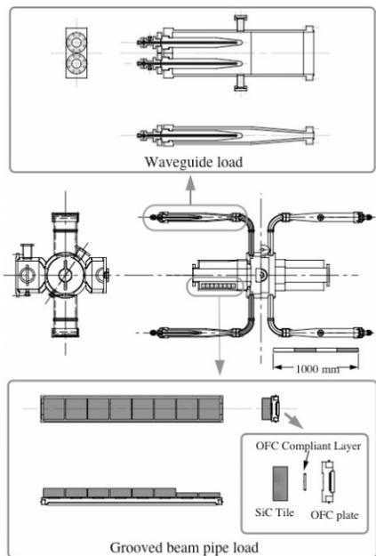
Figure 2: Front and side views of the HOM-damped accelerating cavity part of the KEKB ARES cavity, together with close-up views of the HOM loads.
