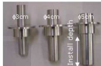
Figure 5: Photograph of slug tuners.
