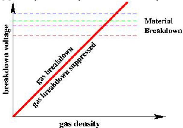
Figure 2: Expected results for material testing of RF cavities. The solid line represents the Paschen curve for a single gas. The dashed lines represent the different materials to be tested.
