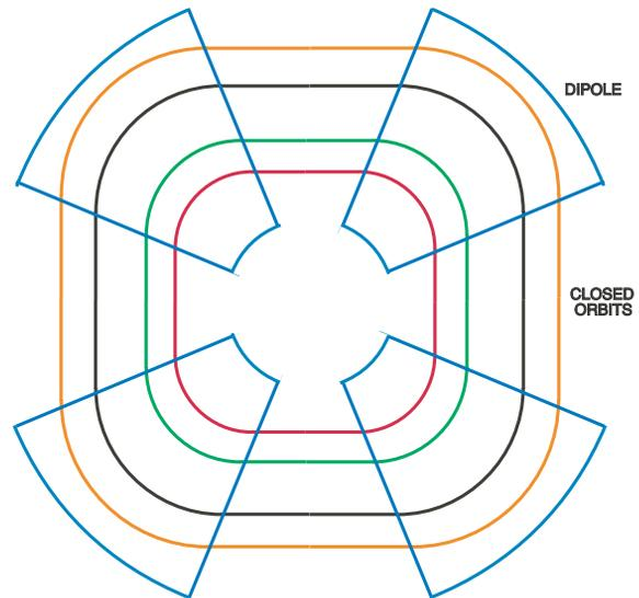
Figure 1: Closed orbits for various beam momenta. Note that positive dispersion results in greater path lengths for higher energy particles.
