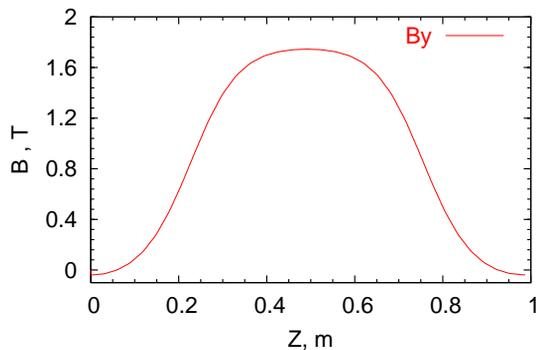
Figure 3: The  $B_y$  component of the calculated dipole field.
