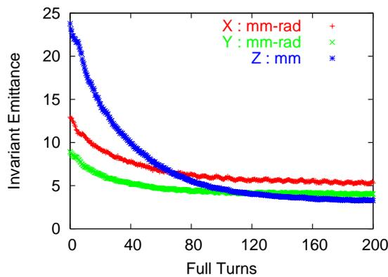
Figure 2: Invariant emittances for each dimension as a function of full turns in the ring.
