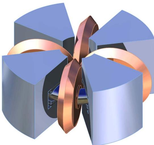
Figure 5: Layout of the cooling ring. The diameter of the cylindrical 201.25 MHz rf cavities is 1.3m
