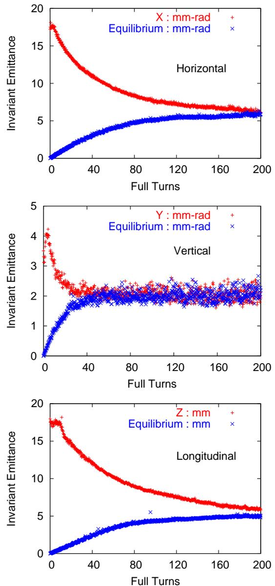
Figure 4: Evolution of invariant emittances for warm and cold muon beams.
