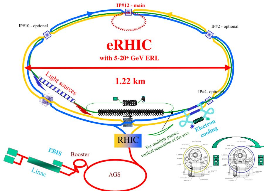
Fig.1. Main layout of ERL based eRHIC with up to four IPs and possible 5 GeV polarized positron storage ring. Polarized electrons are generated at a strained GaAs photocathode, accelerated in a multi-pass ERL, used in one-to-four collisions with the hadrons contra-rotating in the RHIC blue ring, decelerated and finally dumped.
