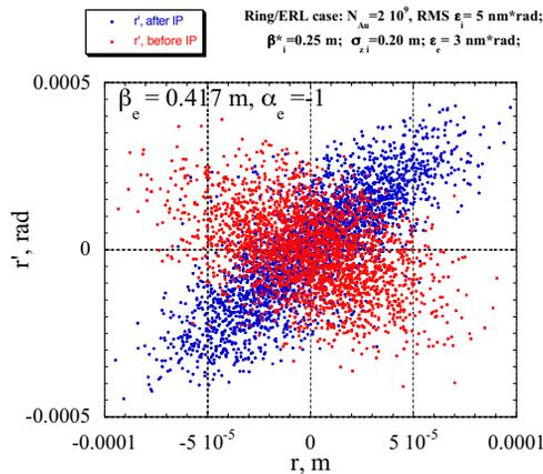
Fig. 2. Round 10 GeV electron beam from ERL with initial transverse RMS emittance of 3 nm<sup>2</sup>rad passes through the IP with the disruption parameter 3.61 (tune shift  $\xi_{xc} = 0.6$ ). The emittance growth is only 11%.
