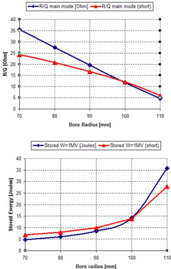
Figure 5: R/Q and stored field energy versus cavity bore.
