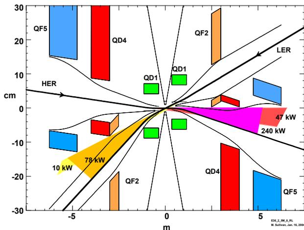
Figure 1. Plan view of the initial Super B-factory IR design. Note the exaggerated vertical scale. The collision angle is  $\pm 14$  mrad. Some additional bending is introduced into the upstream HEB in order to minimize the total beam bending of both beams. The two small horizontal lines inside the QD1 magnets indicate the centerline of each magnet. The detector acceptance of  $\pm 300$  mrad is shown in the middle of the picture.
