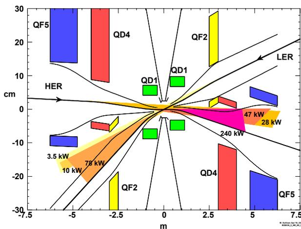
Figure 2. Plan view of the present IR design for a SuperB factory. Note the two extra SR fans generated by the offset QD4 and offset QF2 magnets. The beam pipe design shows a mask present on the incoming HEB side and little or no mask on the incoming LEB side.
