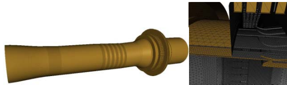
Figure 1: The model of the bellows and its surrounding (Left); the surface mesh of the bellows (Right).
