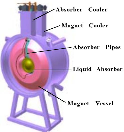
Figure 1. A three-dimensional view of the AFC module.
