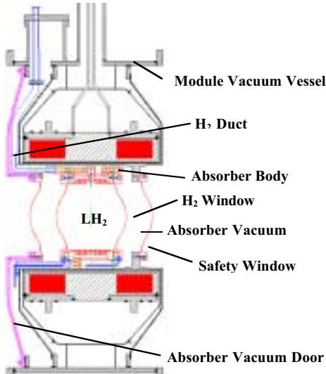
Figure 2: Cross-sectional view of the AFC module showing a liquid absorber for muon ionization cooling.
