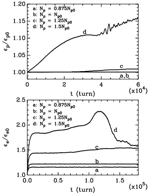
Figure 1: Emittance growth of the  $p$  ( $\epsilon_p$ ) and  $e$  ( $\epsilon_e$ ) beam with different  $p$  bunch intensity  $N_p$ , where  $N_e = N_{e0}$ .  $\epsilon_{p0}$  and  $\epsilon_{e0}$  are the design emittance of the  $p$  and  $e$  beam.
