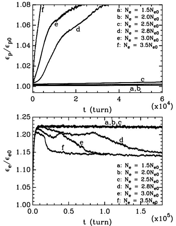
Figure 2: The same as in Fig. 1, but with different  $e$  bunch intensity  $N_e$ . In all the cases,  $N_p = N_{p0}$ .
