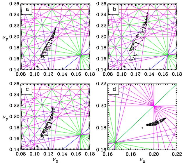
Figure 3: Beam-beam tune spread of the  $e$  beam for (a) case b in Fig. 1 as  $N_e = N_{e0}$  and  $N_p = N_{p0}$ , (b) case d in Fig. 1 as  $N_e = N_{e0}$  and  $N_p = 1.5N_{p0}$ , and (c) case e in Fig. 2 as  $N_e = 3.5N_{e0}$  and  $N_p = N_{p0}$ . (d) The same as (c) but of the  $p$  beam. Solid lines are the even-order resonances up to the 10th order and + indicates the lattice tune.
