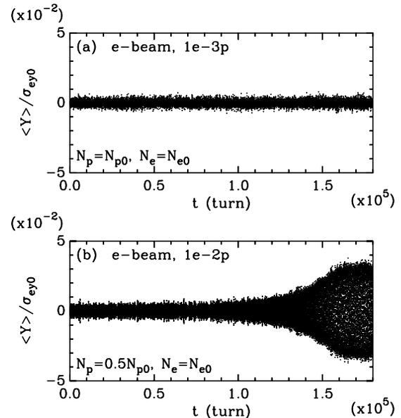
Figure 5: Evolution of the  $e$  beam centroid in the vertical direction. (a) Stable coherent oscillation of case b in Fig. 1 and (b) chaotic coherent oscillation in the case of Fig. 4.
