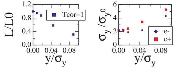
Figure 4: Luminosity and vertical beam size as a function of amplitude of vertical offset noise at the collision point.
