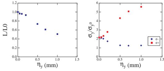
Figure 2: Luminosity and vertical beam size as a function of vertical dispersion at the collision point.
