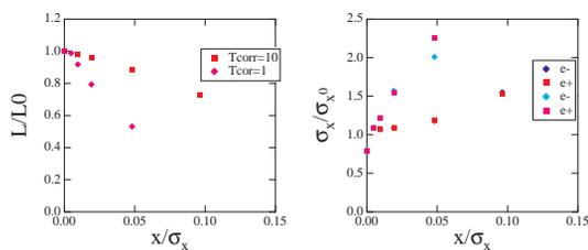
Figure 6: Luminosity and horizontal beam size as a function of amplitude of horizontal offset noise at the collision point.
