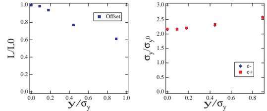
Figure 5: Luminosity and vertical beam size as a function of amplitude of static vertical offset at the collision point.
