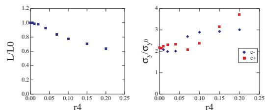
Figure 1: Luminosity and vertical beam size as a function of coupling error,  $r_4$  at the collision point.
