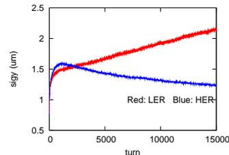
Figure 7: Beam size asymmetry due to different damping time, 4000 and 6000 turns for HER beam, respectively.
