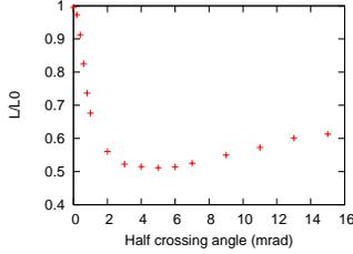
Figure 3: Luminosity as a function of the half crossing angle.
