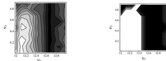
Figure 5: Tune survey results for the dynamic aperture. Left: the dynamic aperture for each tune. The brighter area designates the larger aperture. Right: highlighted area shows the tune space that has larger dynamic aperture than the injected beam
