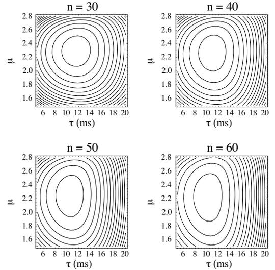
Figure 3: Contour plot of emittance at extraction in  $(\tau, \mu)$  plane, for various number-of-cells  $n$ .
