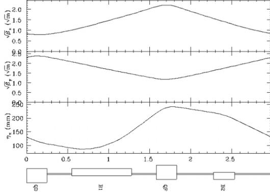
Figure 1: Optics functions of FODO cell with alternating bend. B2 is a reverse bend.
