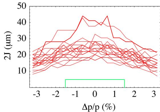
Figure 4: Dynamic aperture of the proposed ring. Thick (red) line is for the case of ideal machine, while thin (red) lines are for the case with machine errors. The (green) rectangular corresponds to the maximum amplitude and energy deviation of injected beam.
