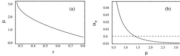
Figure 2: (a): Phase advance per cell that satisfies  $\alpha_p=0$  as a function of  $r$ . (b):  $\alpha_p$  as function of phase advance for fixed  $r$  of 0.5 and  $\theta = 0.314$ .
