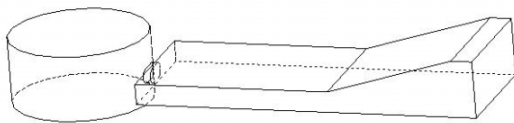
Figure 1: A 3D model of the third cavity coupled to a waveguide through an open iris.
