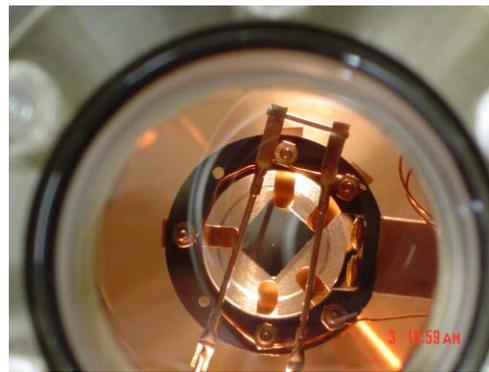
Figure 2: Cathode contacting mechanism in use at Saxet. A similar mechanism is installed in one test chamber at SLAC with a second one to be installed into the polarimeter-equipped chamber at the time of this conference.
