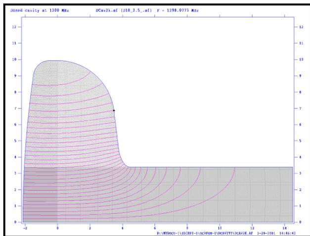
Figure 1, RF Configuration of Single Cell SRF Gun Cavity
