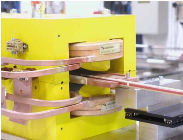
Figure 3: Magnetic measurement with integrating coil of BF magnet
