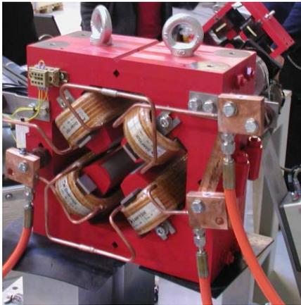
Figure 5: Booster quadrupole magnet.
