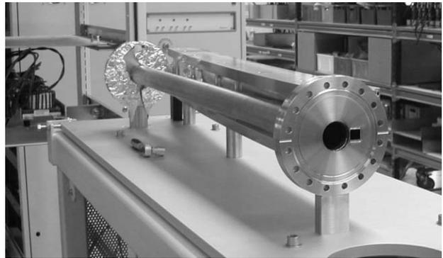
Figure 6: Booster septum magnet with vacuum chamber.
