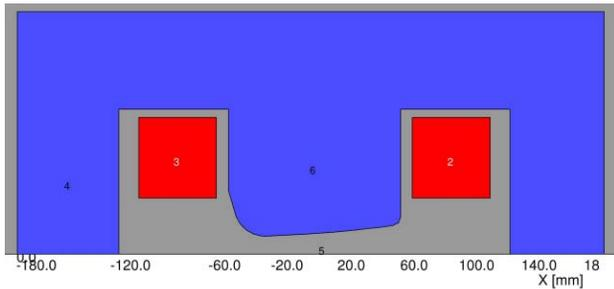
Figure 2: Model of BD magnet showing pole profile
