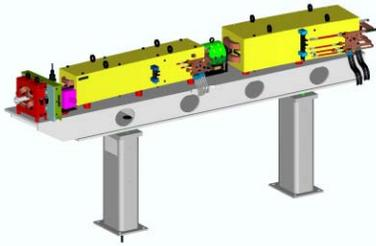
Figure 4: Model of girder with magnets and vacuum chamber. The combined-function BF and BD magnets are yellow, the trim quadrupole red and the trim sextupole green.
