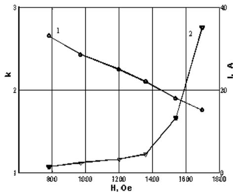
Figure 5: Coefficient of the azimuthal beam inhomogeneity  $k$  (curve 2) and the total beam current  $I$  (curve 1) as a function of the magnetic field amplitude in the vicinity of the Faraday cup.
