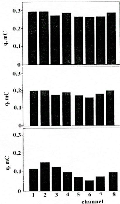
Figure 4: Beam charge distribution  $q$  (mC) along the measuring channels at falling (below), rising (above) and constant magnetic field distribution.
