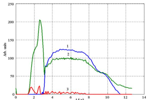
Figure 2: Pulses of voltage (2), beam current (1) and anode current (3), Along the vertical: 1 - 0.4 A/div, 2 - 0.5 kV/div, 3 - 0.04 A/div.
