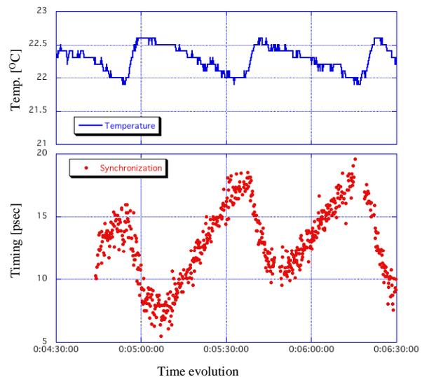
Figure 2: Previous results of the time evolution of the synchronization between the probe laser and the electron beam (lower), and the relevant temperature of the laser room(upper). The frequency of the synchronization is good agreement with that of the temperature.
