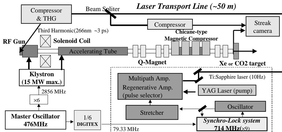
Figure 1: Experimental setup for sub-picoseconds pump- and probe-type radiation chemistry.
