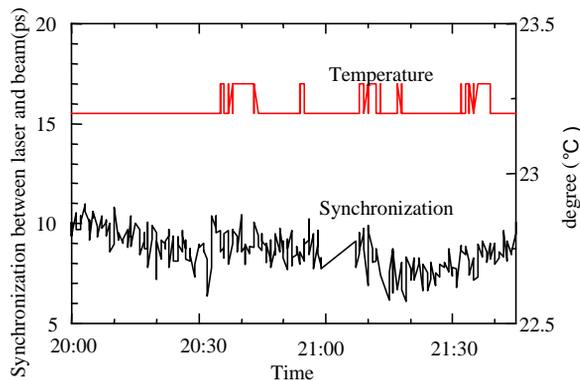
Figure 3: Time evolution of the synchronization and the relevant temperature. The fluctuation of the temperature decreased within 0.1 degrees, and quick and large components in the drift disappears. The jitter in one and a half hours is 600 fs(rms), which is closed to the short time jitter of 340 fs(rms) than previous results (in Fig. 2).
