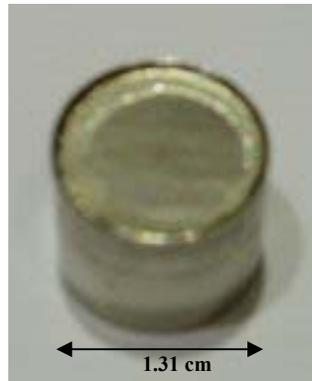
Figure 7: Prototype dispenser cathode.
