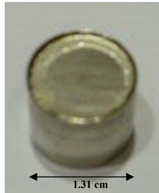
Figure 7: Prototype dispenser cathode.
