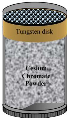
Figure 6 : Dispenser cathode schematic.
