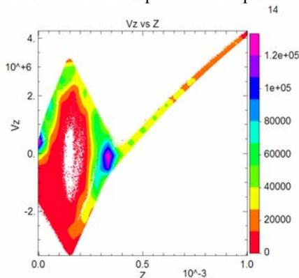
Figure 1. z-vz space showing the structure of virtual cathode downstream of the cathode grid.
