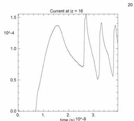
Figure 2. Temporal behavior of the beam current at z=1.5mm from the cathode. The grid-to cathode potential of 30V is turned on over a 2 ns period. The grid to anode potential is 10 KV.
