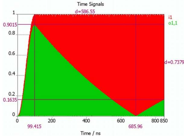
Figure 5: Waveguide input (red) and output (green) signals from MWS time-domain calculations.
