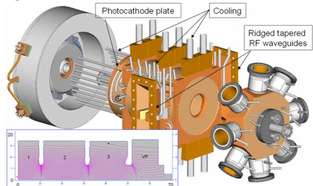
Figure 1: Photoinjector RF cavity with vacuum plenum (VP, right) and emittance-compensating magnets (left).
