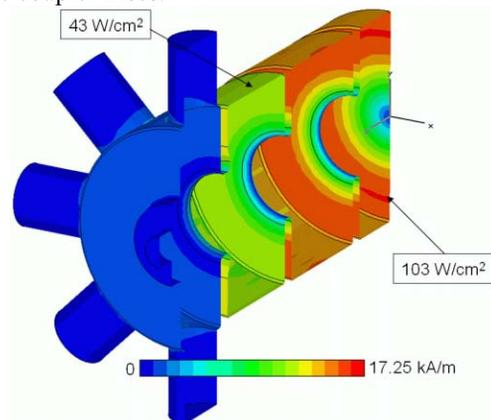
Figure 2: Surface current distribution of the  $\pi$ -mode in the 2.5-cell RF cavity for 775 design (MWS eigensolver).
