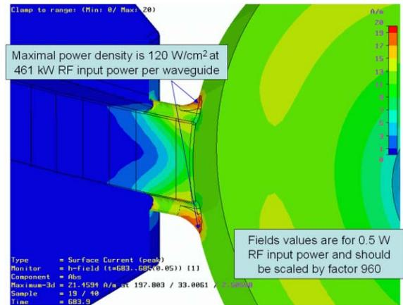
Figure 6: Surface-current distribution near the coupler iris for the matched case. Note the field scale.
