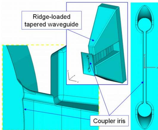
Figure 3: Coupler iris: cut-out view through the middle of the iris gap (left); view from inside the cavity (right).
