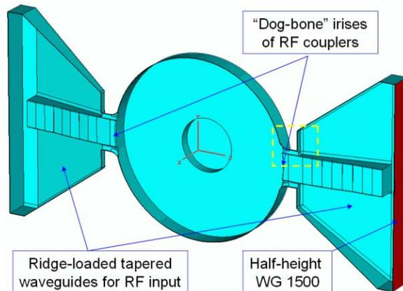
Figure 4: MWS model of RF couplers: a cut-out view through the iris mid-plane, cf. blow-up in Fig. 3 (left).
