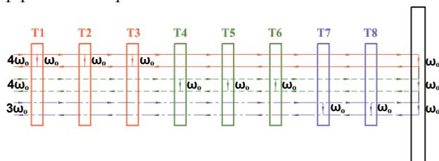
Fig. 5 Schematics of 3 parallel, disk/pipe cooling circuits. The first circuit, represented by solid line (red), cools the first 3 disks and the endplate. The second circuit, represented by dash line (green), cools the next 3 disks and the endplate. The third circuit, represented by dot-dash line (blue), cools the last 2 disks and the endplate.
