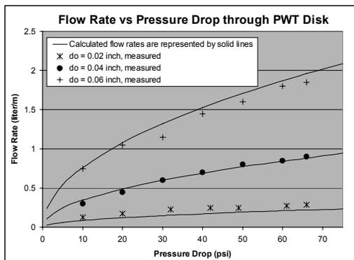
Fig. 3 Disk hydraulic measurements vs calculations.
