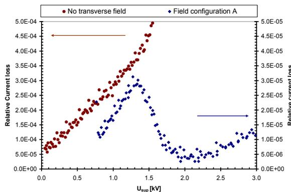
Figure 3: Relative current loss as a function of the suppressor potential with and without transverse magnetic field.  $U_a = 20 \text{ kV}$ ,  $U_{col} = 2 \text{ kV}$ . Note the difference in scale for both data sets. The beam current is  $70 \text{ mA}$  for the case with no transverse field and  $520 \text{ mA}$  for case A.
