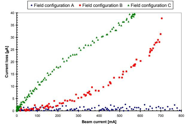
Figure 2: Comparison of the collector efficiency.  $U_a = 20$  kV. Other parameters were chosen to minimize the current loss. For field configuration A and C,  $U_{sup} = U_{col} = 2$  kV. For field configuration B,  $U_{sup} = 0.5$  kV,  $U_{col} = 4.5$  kV.
