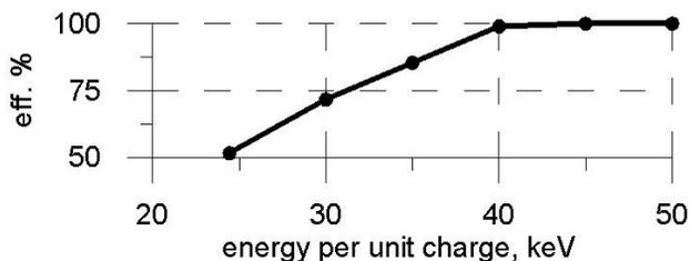
Figure 4. Transmission efficiency. The transmission efficiency is equal to 100% if the energy per unit charge is greater than 45 keV.
