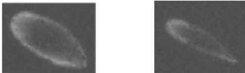
Figure 1. Images of  $\sim 100 \mu\text{A}$   $^{40}\text{Ar}^{7+}$  beam from the NSCL superconducting ECRIS with solenoid focusing. On the left, helium used as a support gas in the source and comprises about 1 emA of the total beam current of 1.8 emA. Shutting off the helium gas supply results in the image on the right; the peak of the argon charge state distribution is 9, so some ring remains.
