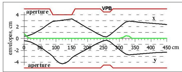
Figure 9. Horizontal (x) and vertical (y) envelopes of the  $^{40}\text{Ar}^{7+}$  ion beam.
