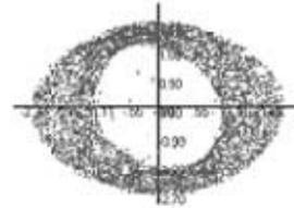
Figure 2. Calculated shape in the  $(x,y)$  plane of  $^{40}\text{Ar}^{7+}$  at a location just after the analysis magnet. With the solenoid, effects of  $Q/A > 7/40$  beams form a ring in  $x-y$  space.
