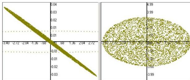
Figure 5. At left is the Ar<sup>7+</sup> ion distribution in  $(x, x')$  plane, on the right the  $(x, y)$  plane is shown.
