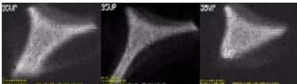
Figure 6: Images of  $^{78}\text{Kr}^{14+}$  beam, first with the sextupole off, next with sextupole on (1.6 kG) but with an incorrect orientation, and last on with the orientation correct.  $V_{\text{ecr}} = 23.82$  kV.
