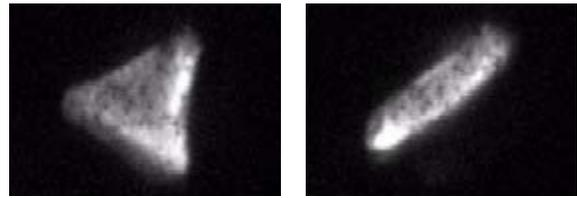
Figure 7: Images of  $^1\text{H}^{+}$  beam, first with the sextupole off and on (0.4 kG) with  $V_{\text{ecr}} = 23.82$  kV. The dispersion plane is rotated left by 45 degrees, so additional quadrupole focusing results in a round image.
