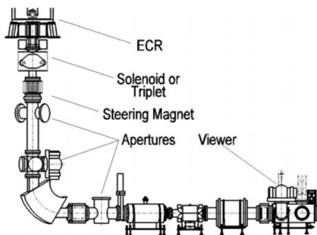
Figure 1: Injection beam line layout. The distance from ECR to analysis magnet is about 2.2 m.
