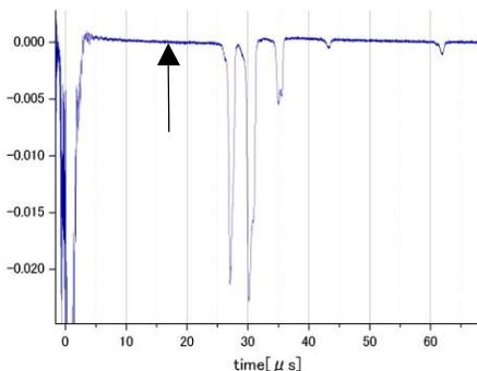
Figure 4: The signal from the detector. In this case, a secondary electron multiplier was used.
