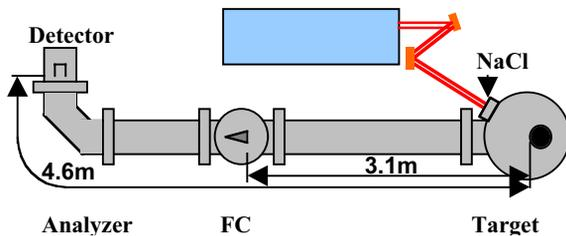
Figure 3: The experimental set up for the plasma measurement.
