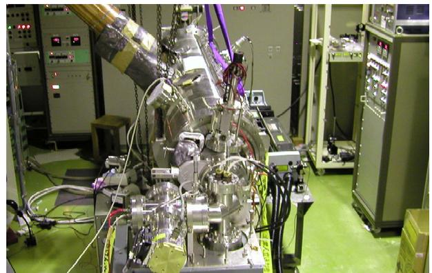
Figure 5: The RFQ and the analyzer.
