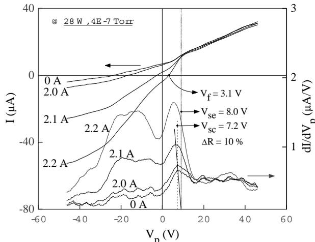
Figure 2: Plasma potential measurement by an EP.
