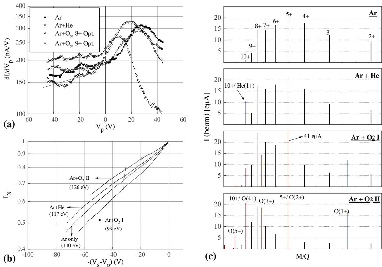
Figure 3: Langmuir probe measurements of (a) plasma potentials, and (b) fast electron temperatures; and (c) corresponding external beam charge distributions (CSD's) for pure Ar, He gas mixed and O<sub>2</sub> gas mixed plasmas.
