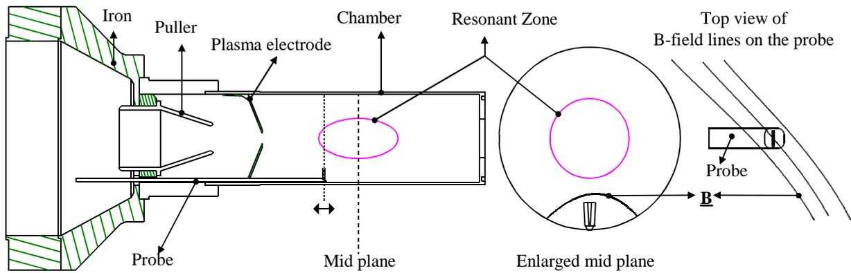
Figure 1: The probe positioning relative to the radial loss cones of the magnetic structure of CAPRICE ECRIS.
