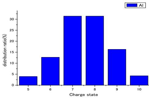
Figure 2: Charge state distribution (Al).
