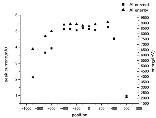
Figure 6: Current change by focus position (Al).
