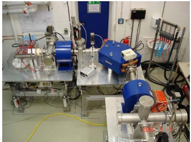
Figure 6: Top view of ECR ion source with LEBT.
