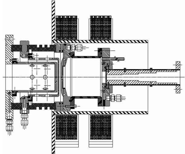
Figure1: The source design used at ACCEL.
