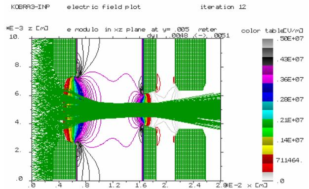
Figure 2: Simulated extraction of deuteron beam.
