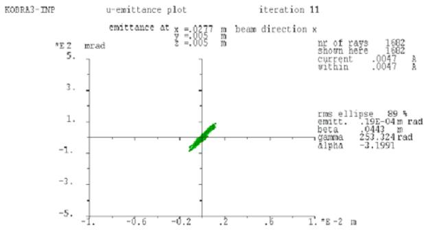
Figure 3: Emittance of simulated deuteron beam.
