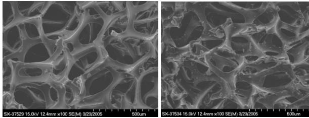
Figure 2: Scanning Electron Micrographs of 4xRVCF (left) and 6xRVCF (right).
