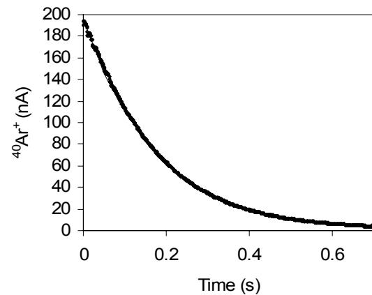
Figure 3: Effusive-flow spectrum of  $^{40}\text{Ar}$  in the serial-coupled vapor transport system.
