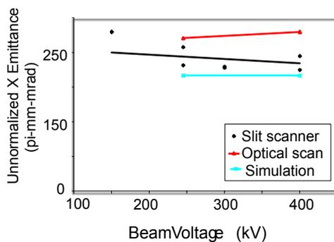
Figure 6: Comparison of the measured unnormalized x emittance and the same emittance predicted by simulation.
