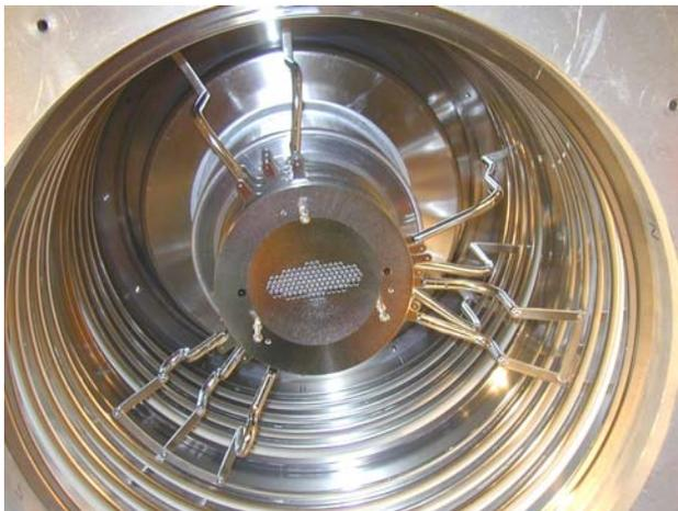
Figure 2: Einzel Lens Assembly installed in the top of the column (without the field shield installed).
