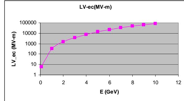
Figure 1: Product of L in meters and corrector cavity voltage in MV as function of energy.
