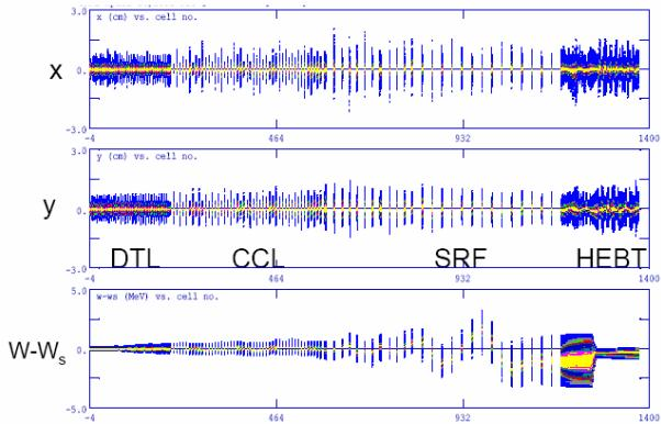
Figure 5: Beam envelopes through the SNS linac and HEBT.
