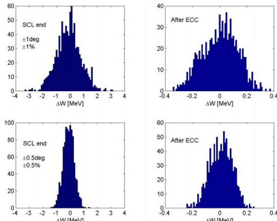
Figure 4: Histograms of beam centroid energy at the end of the linac and after the ECC for the two sets of rf control.
