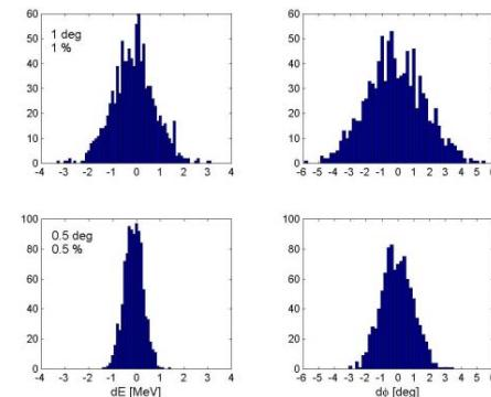
Figure 2: Histograms of beam centroid energy and phase jitters at the end of linac for  $\pm 1^\circ$  and  $\pm 1\%$  rf phase and amplitude control (upper plots) and for  $\pm 0.5^\circ$  and  $\pm 0.5\%$  rf phase and amplitude control.
