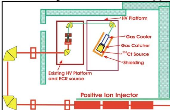
Figure 2: Schematic overview of the proposed  $^{252}\text{Cf}$  fission fragment beam facility. An existing ECR ion source will be modified for charge breeding and then inject these beams into the ATLAS linac.
