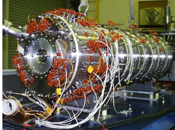
Figure 4: The assembled RIA prototype gas catcher as seen from the nozzle/RF cone end. A shorter version of this device will be used for this project.
