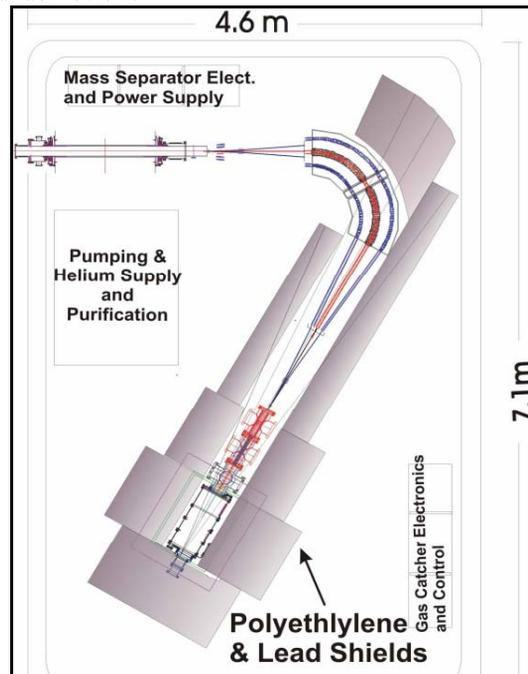
Figure 6:  $^{252}\text{Cf}$  fission source and gas catcher beam transport shielding plans on the HV platform.
