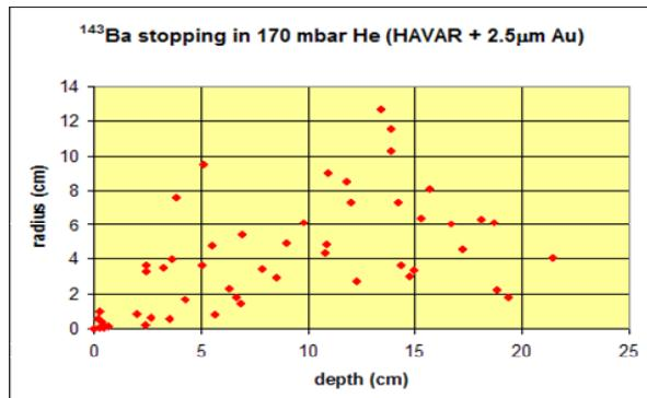
Figure 3: Distribution of stopping positions for  $^{143}\text{Ba}$  fission fragments in 170 mbar He.
