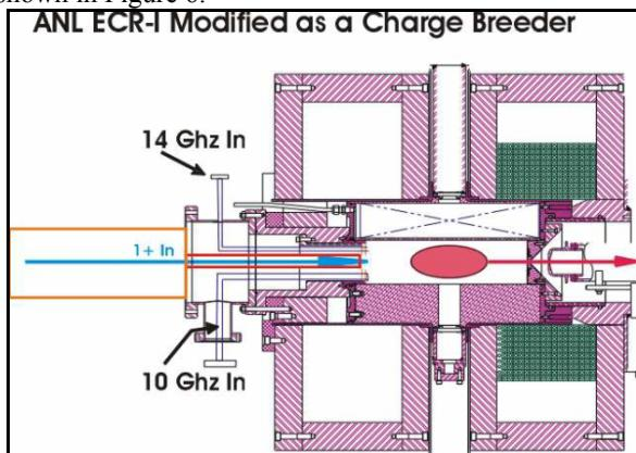
Figure 5: 10 & 14 GHz ECR-I ion source modified on the injection side for charge breeding operation.
