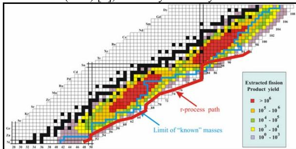
Figure 1: Distribution of fission products from the spontaneous fission of  $^{252}\text{Cf}$ . The color code gives the extracted low-energy ion beam intensity ( $\text{s}^{-1}$ ) for a 1 Curie source.
