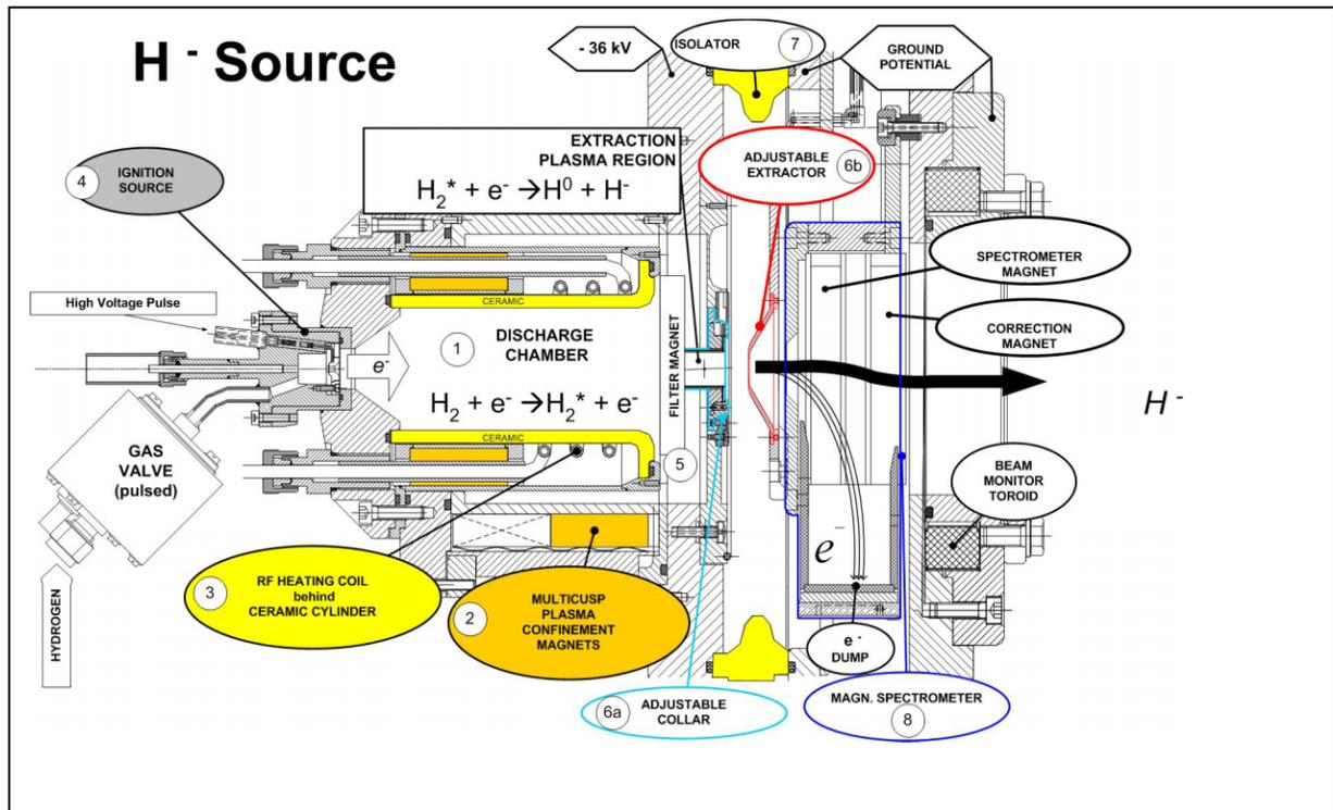
Figure 1: DESY HERA Volume H<sup>-</sup> Source.
