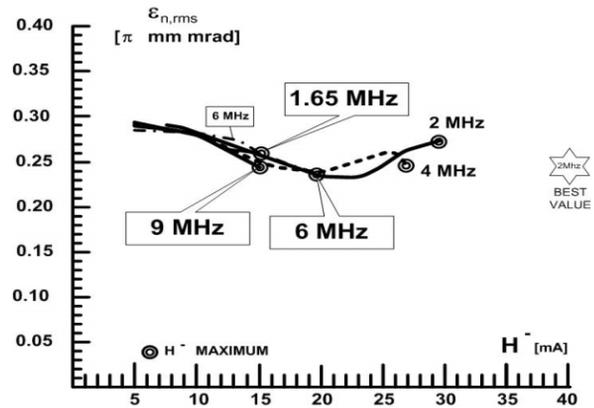
Figure 3 : Frequency and H<sup>-</sup> current dependence of the rms emittance.
