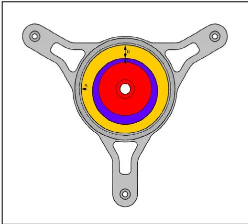
Figure 2 : Extractor electrode horizontal and vertical adjustable by eccentric rings.
