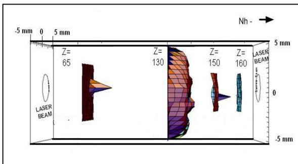
Figure 4: 3D H<sup>-</sup> intensities measured with photodetachment.
