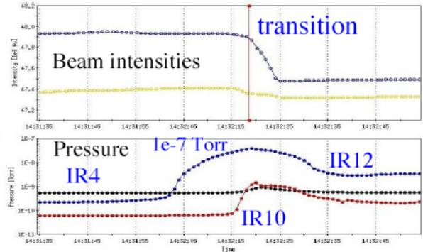
Figure 3 Beam intensity and pressure at IRs, the pressure rise occurs before the major beam loss.
