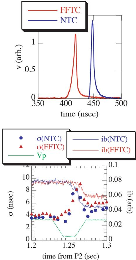
Figure 1 (a) Output of the fast bunch monitor at t=1.25 sec. (b) RMS bunch length, beam intensity and programmed-voltage around the transition energy.
