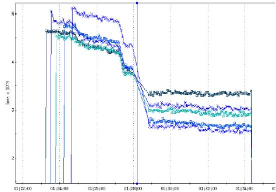
Figure 2 Electron-ion instability induced loss: the first/last bunches have loss of (13/70%).
