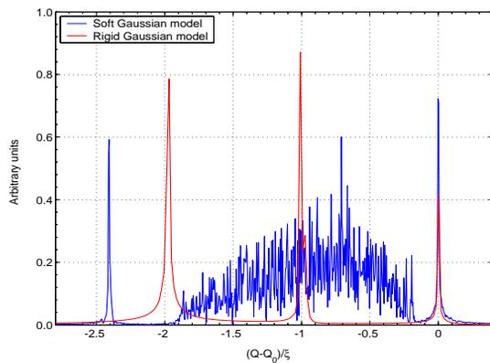
Figure 2: Tune spectra of rigid bunch (red line) and soft Gaussian bunch (blue line) coupled by two head-on collisions in IPs 1 and 3 in a fourfold symmetry.
