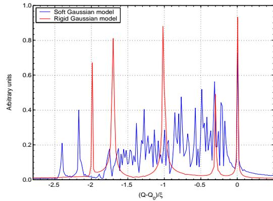
Figure 1: Tune spectra of rigid bunch (red line) and soft Gaussian bunch (blue line) coupled by two head-on collisions in IPs 1 and 2 in a eightfold symmetry.
