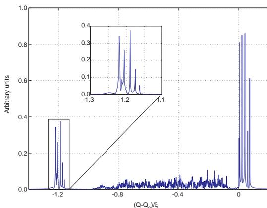
Figure 3: Tune spectrum of a train of 6 soft Gaussian bunches coupled by one head-on collision in IP 1 and one long range interaction in IP 5.
