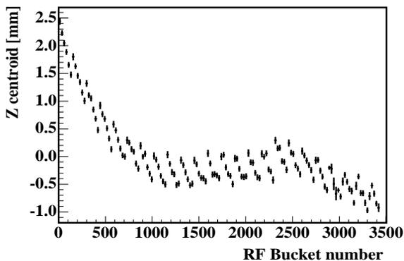
Figure 2:  $z_c$ -variation along the bunch train. The sharp transition at the beginning of the train reflects the RF-phase jumps caused by the 2% abort gap. The periodic structure is caused by variations in relative RF phase associated with the short gaps between the minitrains. The drift-chamber time resolution is sufficient to resolve individual bunches.
