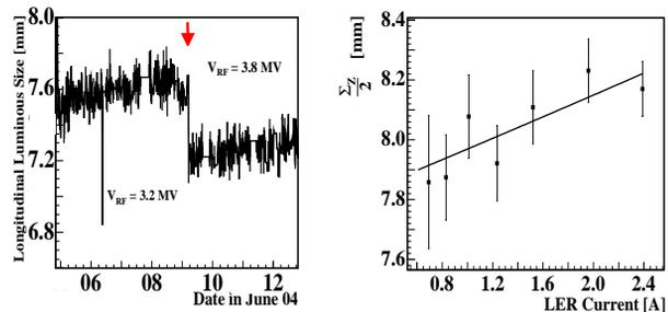
Figure 3: Left: history of the r.m.s. luminous length  $\sigma_z^L$ , before and after the LER RF voltage  $V_{RF}^+$  was increased (arrow). The HER RF voltage  $V_{RF}^-$  remained constant. Right:  $e^+$ -current dependence of the fitted value of  $\Sigma_z/2$  ( $\approx \sigma_z^L$ ) measured during a long coast-down. The line shows the fitted current-dependence (see text). The HER bunch length and the  $\beta$  functions are fixed in the fit.
