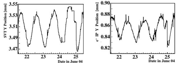
Figure 1: Time history of the vertical IP position. Left: vertical luminous centroid reported by *BABAR*. Right:  $y$  position of the  $e^+$  beam at the IP, measured by the BPM's. The sine-like behavior is caused by day-night temperature variations.
