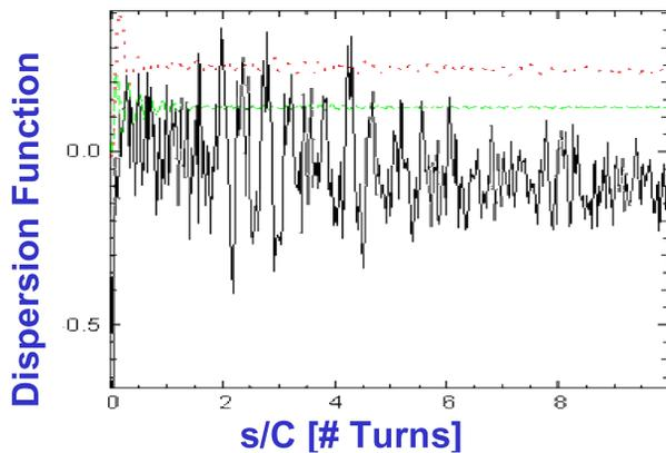
Fig. 4: Dispersion function for  $\delta=5e-5$  [black], 0.001 [red], and 0.01 [green] velocity spreads, and  $I=24$  mA.
