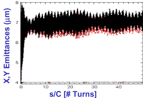
Fig. 5: Effective unnormalized emittance with (black) and without (red) the Earth field for  $I=0.6$  mA and  $\delta=0.01$ .
