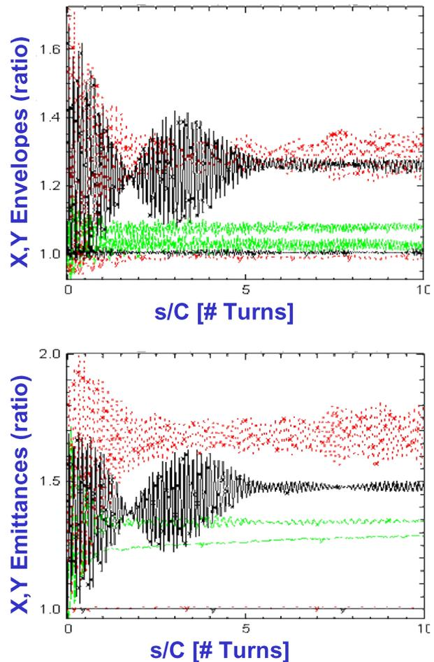
Fig. 2: (a) rms beam radius, and (b) rms emittance for the same three cases in Fig. 1.
