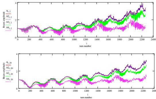
Figure 1: Multi-particle simulation results with 1000 particles under the influence of a resistive wall wake of  $8.7 \times 10^5$   $\xi = 1.87$  with total charge equal to  $260 \times 10^{11}$  protons. Top graph is head of bunch ( 4 nsec from center) and bottom is tail ( 4 nsec from center). Top two traces are the beam envelope with  $\xi_1 = 0$  and  $\xi_1 = .422$  (no real difference), middle trace  $\xi_1 = .844$  and bottom trace  $\xi_1 = 1.26$
