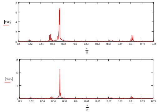
Figure 2: Fourier spectrum from a multi-particle simulation results with 1000 particles with total charge equal to  $260 \times 10^{11}$  protons and  $\xi = 1$  and  $\xi_1 = 1.2$ . Top graph is under the influence of a resistive wall wake of  $8.7 \times 10^5$  bottom graph is under the influence of wake  $4.7 \times 10^5$ . the ratio between the largest off tune peak for the larger wake field is 0.18 and 0.07 for the smaller wake
