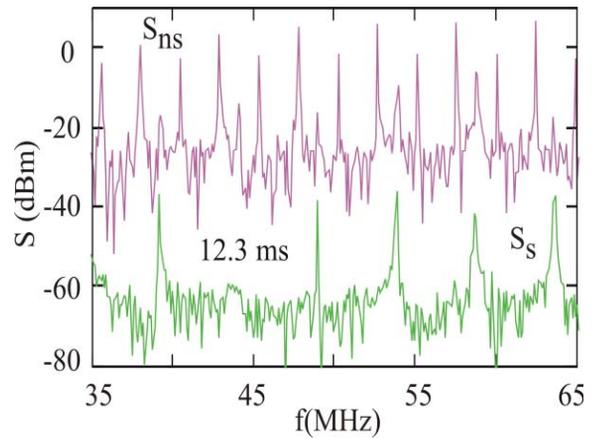
Figure 4: Pie electrode spectra with ( $S_s$ ) and without ( $S_{ns}$ ) PM, where  $S_s=S-10$  dB and  $S_{ns}=S+40$  dB, at  $t=12.3$  ms.
