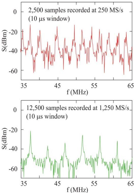
Figure 3: Aliased (top) and clean (bottom) spectra
