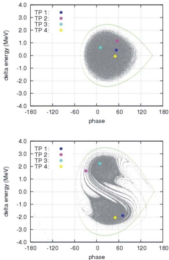
Figure 3: CAPTURE\_SPC phase-space plot before and after the introduction of PM, the PM amplitude is  $4.3^\circ$ .
