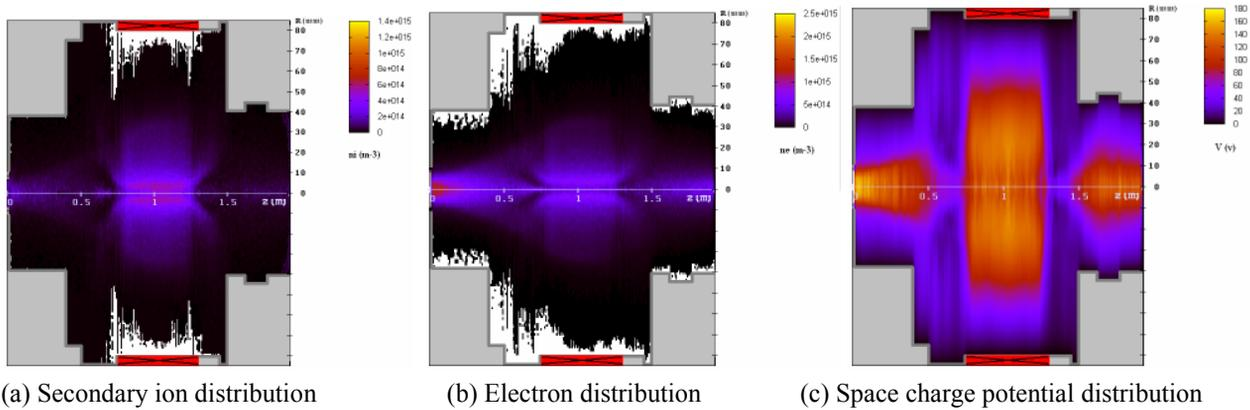
(a) Secondary ion distribution      (b) Electron distribution      (c) Space charge potential distribution
