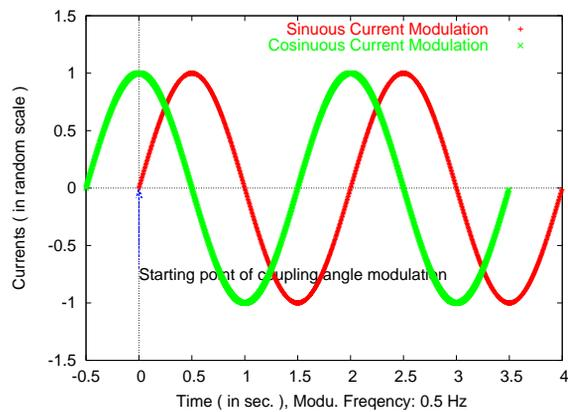
Figure 2: Skew quadrupoles' Currents in the operational coupling angle modulation
