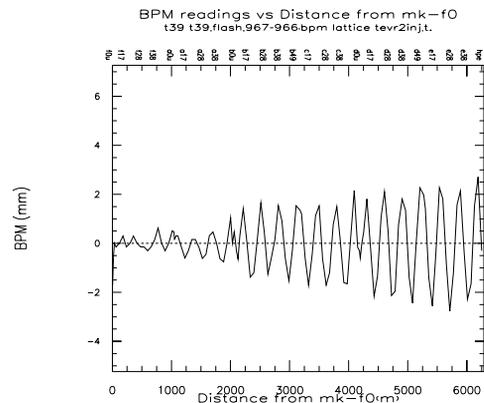
Figure 1: Vertical orbit data displaying growth of amplitude along the Tevatron circumference.
