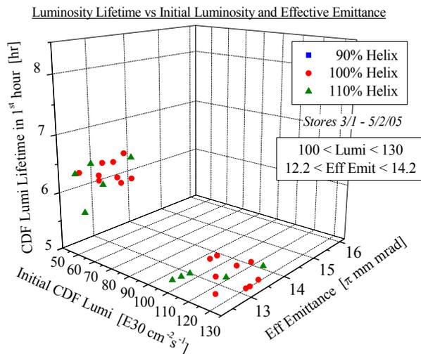
Figure 3: Luminosity lifetime in the first hour for the CDF experiment as a function for a specific set of initial luminosities and effective emittances; only projections onto two planes are shown. No 90% helix stores are in this population of stores.
