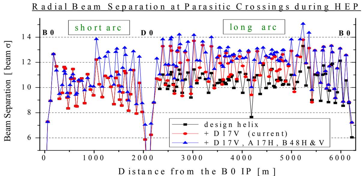
Figure 1: Separation between protons and antiprotons at all parasitic crossings for the design separator configuration (black squares), with the addition of vertical separators at the D17 location (red circles), and with all proposed additional separators (blue triangles).
