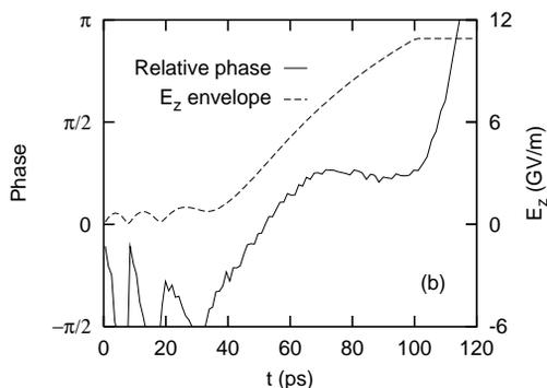
Figure 2: Evolving phase difference and  $E_z$  for the CO<sub>2</sub> laser parameters of Fig. 1. For  $t$  between 60 and 100 ps there is a constant phase difference between the lasers and accelerating field, permitting control of electron injection.
