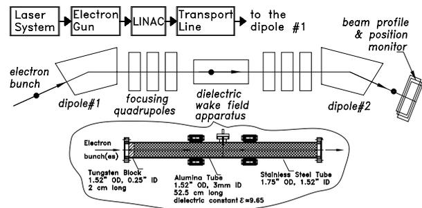
Figure 3: Schematic of the experimental setup and the dielectric wake field apparatus (DWA).
