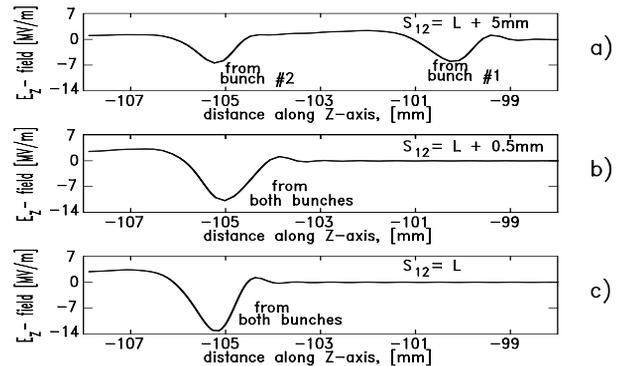
Figure 2: The  $E_z$  - field profile on the DWA axis with different bunch spacing  $S_{12}$ . (a)  $S_{12} = L + 5\text{mm}$ , (b)  $S_{12} = L + 0.5\text{mm}$ , (c)  $S_{12} = L$  (the wake-field period  $L=0.21022\text{m}$ ,  $A=1.5\text{mm}$ ,  $R=19.31\text{mm}$ , and  $\epsilon = 9.65$ ; charge/ bunch is 1nC). Constructive superposition occurs when  $S_{12}$  is close to  $L$  (or, in general, to  $JL$ , where  $J$  is any integer).
