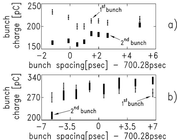
Figure 5: Charges of the 2<sup>nd</sup> and 1<sup>st</sup> bunches [the accuracy a)  $\approx \pm 3\%$ , and b)  $\approx \pm 5.5\%$ ]. The difference in bunch energy losses is shown in Fig.4.
